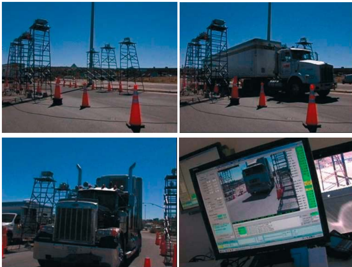
Fig. 6. Remote sensing examinations of trucks
